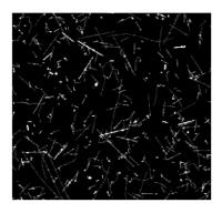
Illustration of single particle sensitivity of Timepix device. The tracks of different particles of radiation background (mostly muons and few protons) were recorded in 5 minutes on board of airplane. No noise (clean zero) is seen in dark regions.
