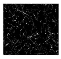
Illustration of single particle sensitivity of Timepix2 detector. The tracks of different particles of radiation background (mostly muons and few protons) were recorded in 5 minutes on board of an airplane. No noise (clean zero) is seen in the dark regions.
