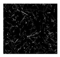
Illustration of particle tracking capability of Timepix3 device: The tracks of different particles of radiation background were recorded during 10 minutes in office space in Prague. Brightness corresponds to energy. No noise (clean zero) is seen in dark regions. All basic particle track types are seen nicely: muons = straight lines, alpha particles = bright balls, electrons = curved lines, gamma and X-rays = dots and blobs.
