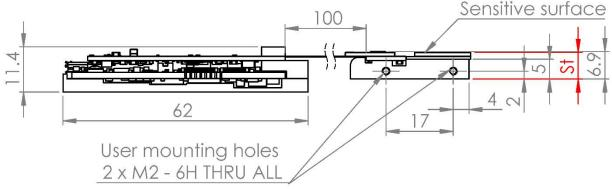
All dimensions are in mm. The sensor specific dimensions  $s_t$  and  $s_w$  (shown in red) are listed in the following table.
