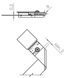
Bending radius according to IPC-2223 standard (2 layers flex PCB, 0,2 mm thick)
