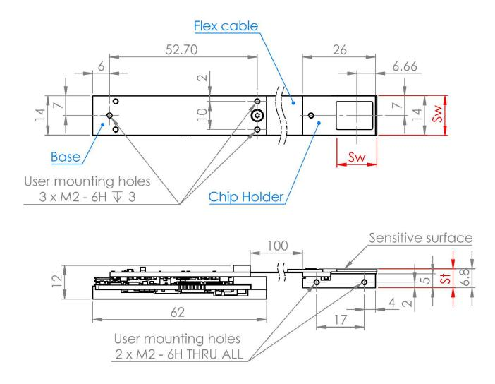
All dimensions are in mm. The sensor specific dimensions  $s_t$  and  $s_w$  (shown in red) are listed in the following table.
