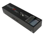
Timepix 3 Si or CdTe 55 x 55 um 2.35 Million hits/s USB 2.0 (High-Speed) 80 x 21 x 14 mm 30 g
