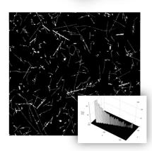
Illustration of single particle sensitivity of Timepix3 device. The tracks of different particles of radiation background (mostly muons and few protons) were recorded in 5 minutes on board of airplane. No noise (clean zero) is seen in dark regions. Inset shows the time profile along one muon track.
