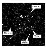
Illustration of particle tracking capability of Timepix3 device: The tracks of different particles of radiation were recorded during 10 minutes in normal office space in Prague. Brightness corresponds to energy. No noise (clean zero) is seen in dark regions. All basic particle track types are seen nicely: muons = straight lines, alpha particles = bright balls, electrons = curving lines, gamma and X-rays = dots and blobs.
