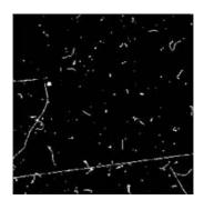
Illustration of single particle sensitivity of Timepix device. The tracks of different particles of normal radiation background were recorded in 10 minutes. No noise (clean zero) is seen in dark regions.
